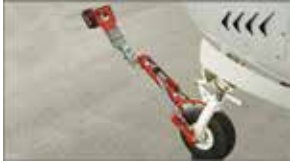
Sidewinder attached securely to the front wheel.
