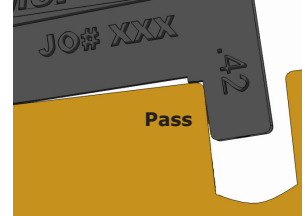
3. If the step touches the rail, lifting the gauge up, the wear is less than 0.42. If the step does not touch the rail, the wear is more than 0.42 and the seat rail must be replaced.
