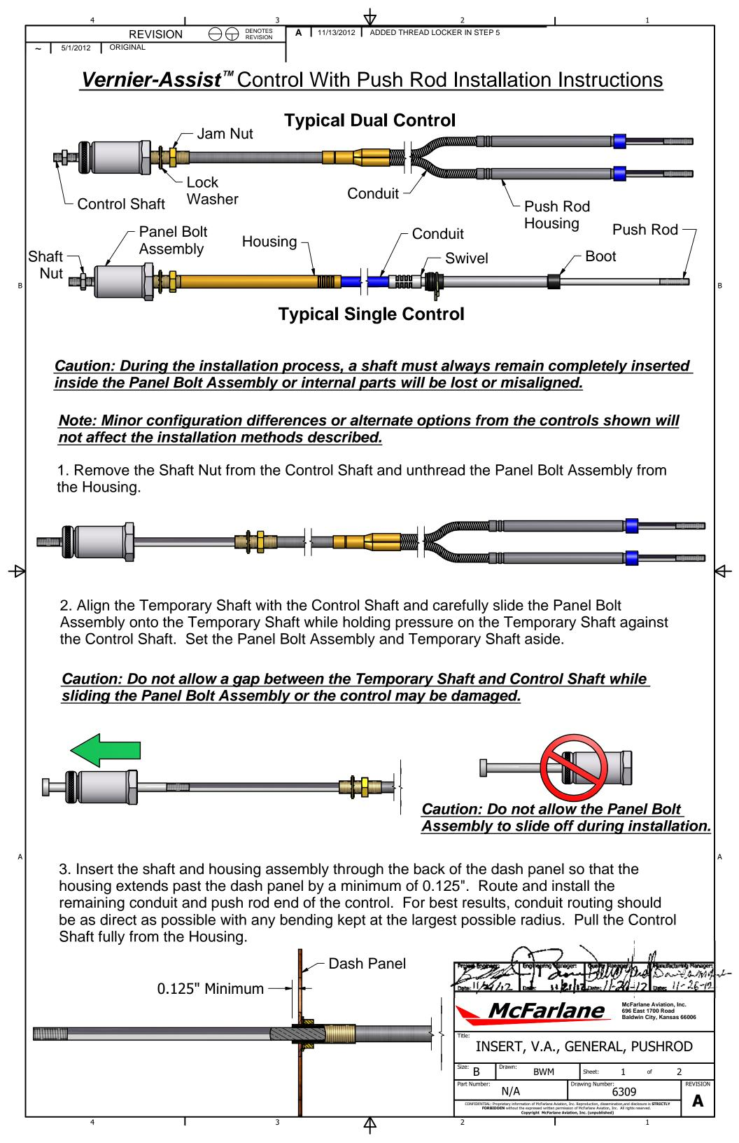
4. Align the Temporary Shaft with the Control Shaft and carefully slide the Panel Bolt Assembly back onto the Control Shaft. Do not allow the Control Shaft to slide back into the Housing while performing this operation. Thread the Panel Bolt Assembly onto the Housing (~3 full turns) and tighten the Lock Washer and Jam Nut until the Panel Bolt Assembly is secure against the Dash Panel.
