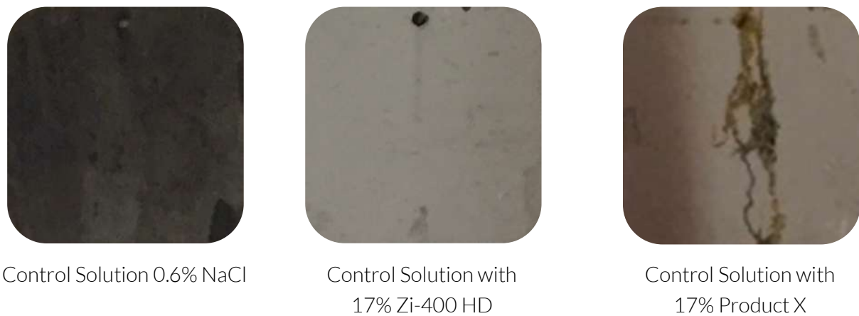
Figure 9. Specimens of SAE 4140 steel after immersion for 30 days in 0.6% NaCl solution (Control) with and without Zi-400 HD or Product X.
