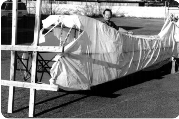
This simple fuselage turning jig makes covering your fuselage much easier.
