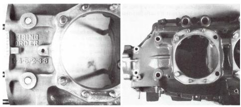
Figure 2-38. Anchored through-stud on top, body-fit through-stud on bottom.
