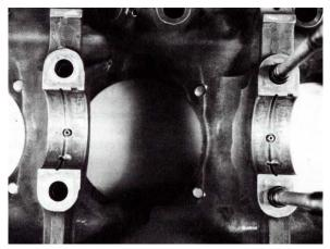
Figure 2-39. Anchored through-stud design showing dowels surrounding protruding throughstud on one side and dowel boss on the other. Dowels provide rigidity to crankcase preventing movement between the surfaces. Dowels must fit tight to prevent oil leakage out past through-studs.
