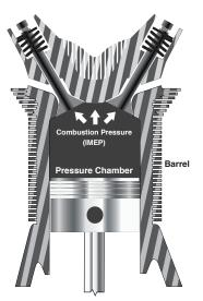
Figure 2-34. Cylinder is a cap to a pressure vessal.
