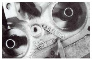
Figure 2-35. 10-520 cylinder showing casting revision number.
