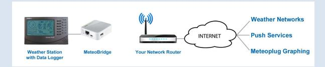
MeteoBridge is a low power Wi-Fi enabled router, running the MeteoBridge software created by SmartBedded, which sends your data to where you want it without running a PC 24/7.
