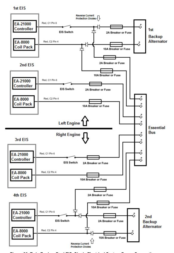
Figure 20: Twin Engine, Dual EIS, Single Electrical System Power Connections
