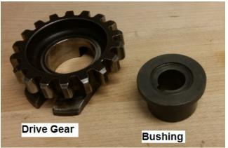
Figure 8: Magneto Drive Gear and Bushing
