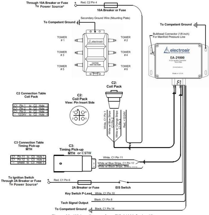
Figure 22: Wiring diagram for a EIS-61000 Series Kit
