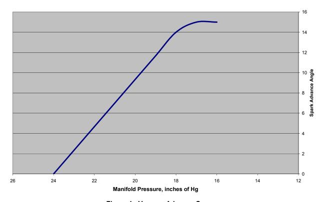
Figure 1: Vacuum Advance Curve
