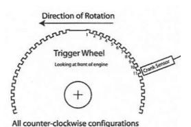
Figure 6: Crank Shaft Trigger Wheel Positioning
