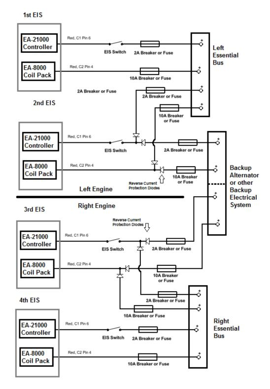
Figure 21: Twin Engine, Dual EIS, Dual Electrical System Power Connections
