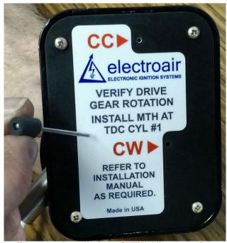
Figure 7: Installation of MTH Alignment Pin
