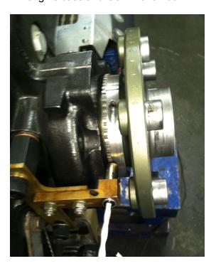
Figure 4: Typical installation of CSTW on a Lycoming 540 engine. Picture shows orientation of trigger wheel and typical bracket location. Please contact Electroair Tech Support if there are any questions about the assembly.
