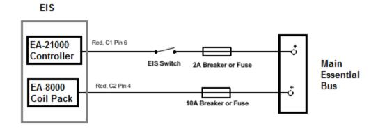
Figure 17: Single Engine, Single EIS Power Connection
