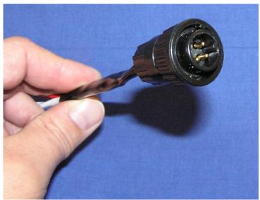
Figure 16: Coil Pack Harness Plug
