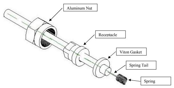
Figure 14: Spark Plug Wire Component Stack Up.
