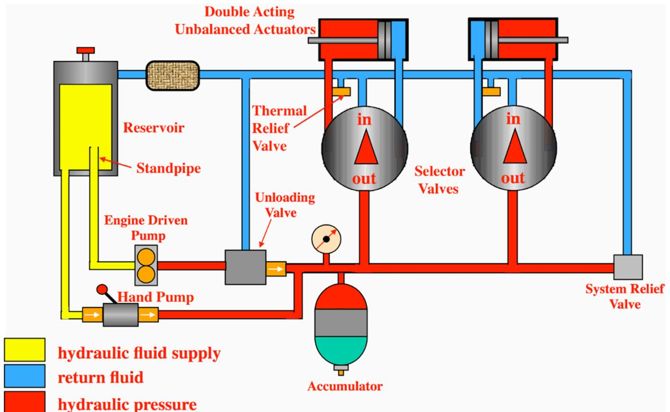
Figure 7-12. Small airplane hydraulic system.
