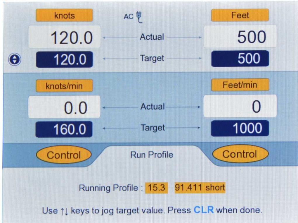
**Figure 3.44 : Run Profile (Jog Pitot Target at 15.3)**
