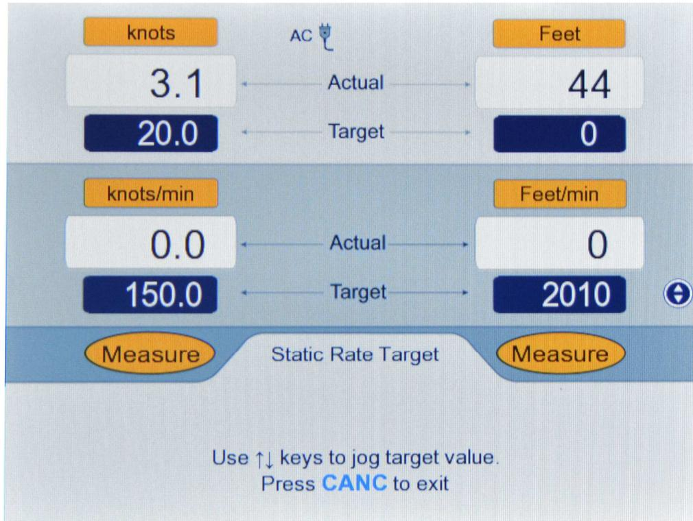
**Figure 3.14 : Jog the Static Rate Target value**
