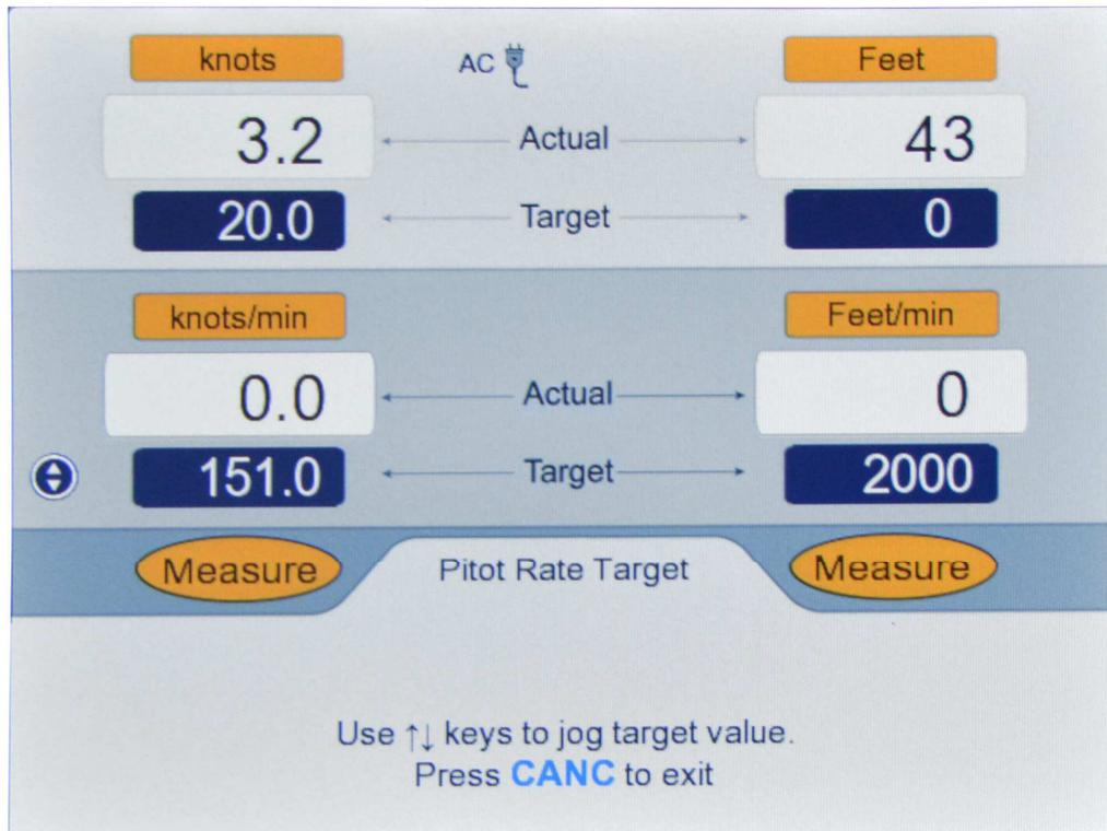
**Figure 3.12 : Jog the Pitot Rate Target value**
