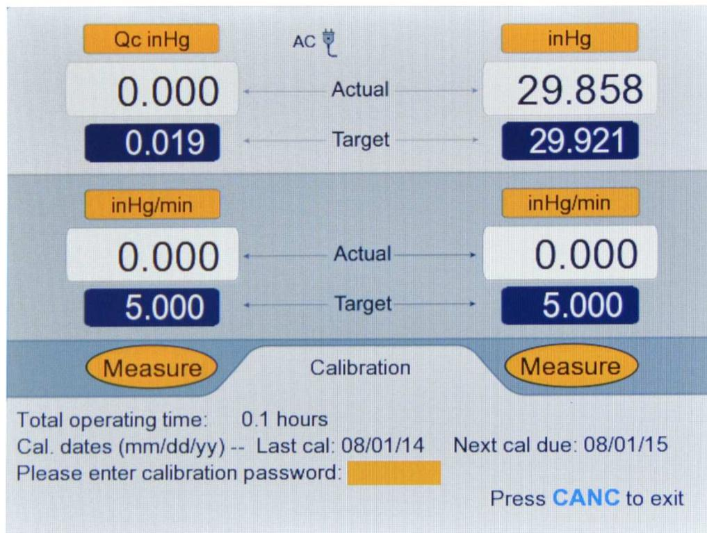
**Figure 6.2 : Calibration (password)**
