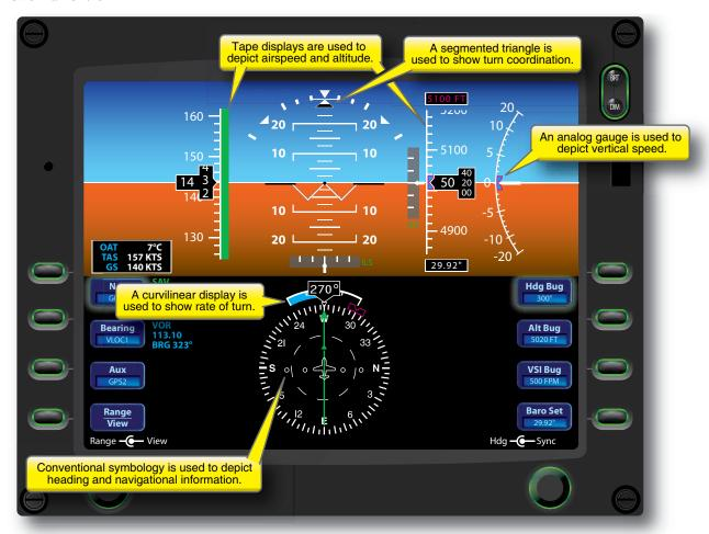
Figure 2-1. A typical primary flight display (PFD).
