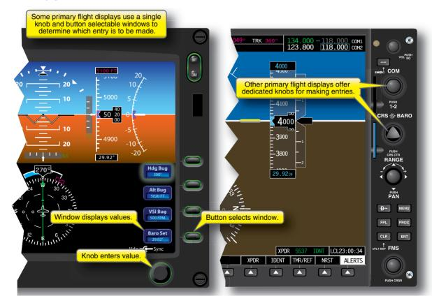
**Figure 2-6.** *Making entries on a PFD.*
