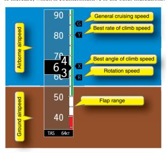
**Figure 2-2.** *Vertical airspeed (tape type) indicator.*
