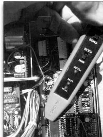
*Logic probe to trace digital circuits.*
