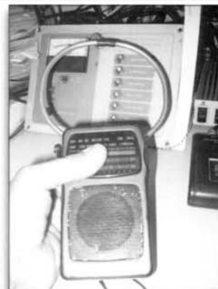
*Simple AM radio with added loop antenna for sniffing RFI from a voltage panel.*
