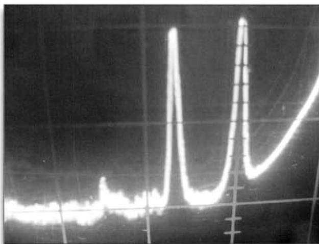
*Oscilloscope measuring a two-tone test on an aircraft SSB.*
