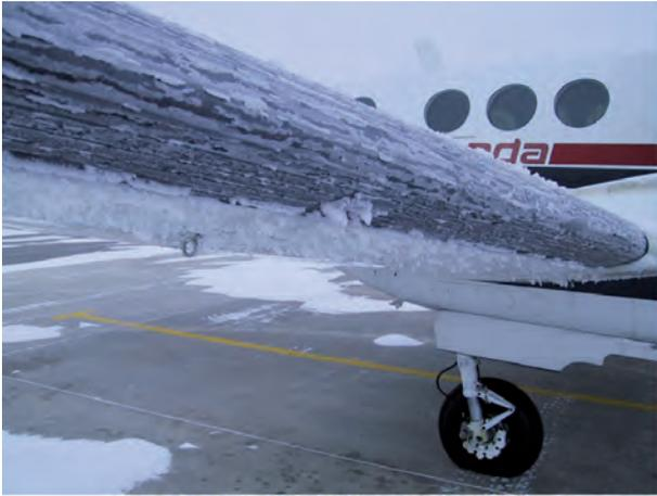
Figure 16.3a: Removal of rime ice by the wing boot.
