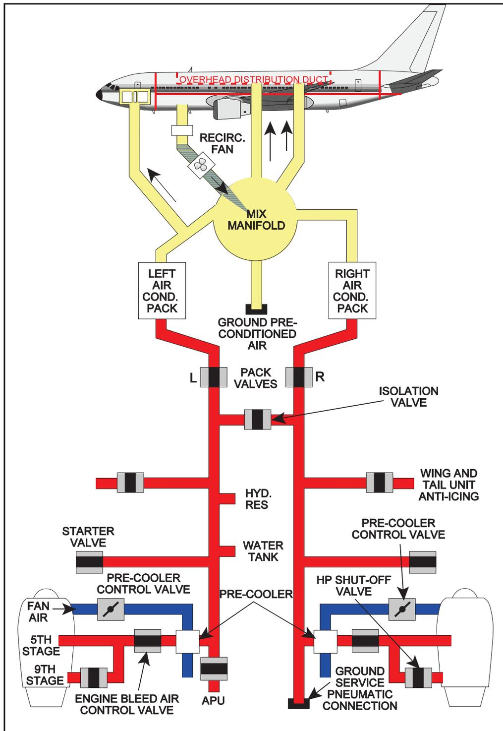
Figure 10.1a: Air sources and uses (schematic).
