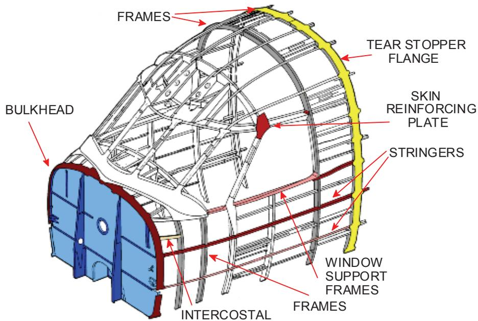
Figure 1.5: Damage tolerant structure.
