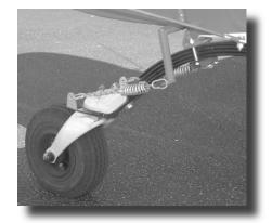
Figure 1. Tail wheel assembly (Aviat Husky). Pulling the stick back to your gut makes steering more effective.
