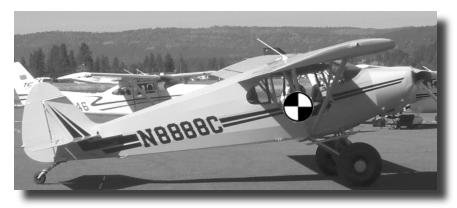
Figure 5. The side view of the taildragger reveals a lot of side area behind the main gear. The cg is behind the main gear.
