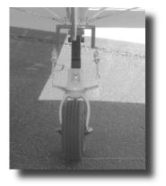
Figure 2. Pay particular attention to the springs during the walk-around inspection checking alignment and security.
