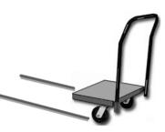
Figure 4. Tricycle-gear airplane comparison. With the mass ahead of the main wheels (this comparison has a person pulling the hand cart), the tricycle-gear airplane tracks straight during takeoff.
