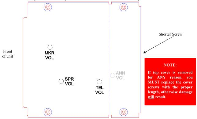
Figure 2-3- PMA8000C Adjustments, top cover
