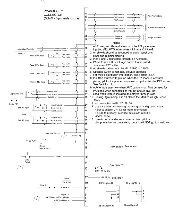
PMA8000C Audio Selector Panel and Intercom System Installation and Operator's Manual
