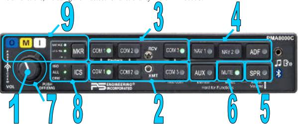
Figure 3-1 PMA8000C Operating Controls
